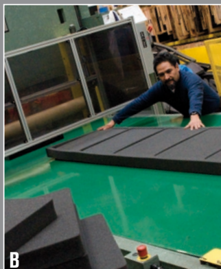
Your layout is then transferred to your choice of foam to be cut using either (A) Water Jet Technology, (B) Die Cut Technology or (C) CNC router technology.
