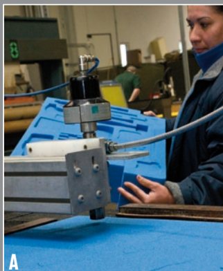
Your layout is then transferred to your choice of foam to be cut using either (A) Water Jet Technology, (B) Die Cut Technology or (C) CNC router technology.
